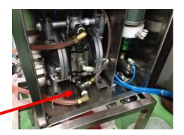
After loosening round bolt by hand, Only sliding pump, can detach pump very easily.
